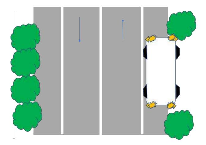
Properplacement of a Type AMultifunction and Small Capacity Vehicle on a roadway when loading and unloading students.
