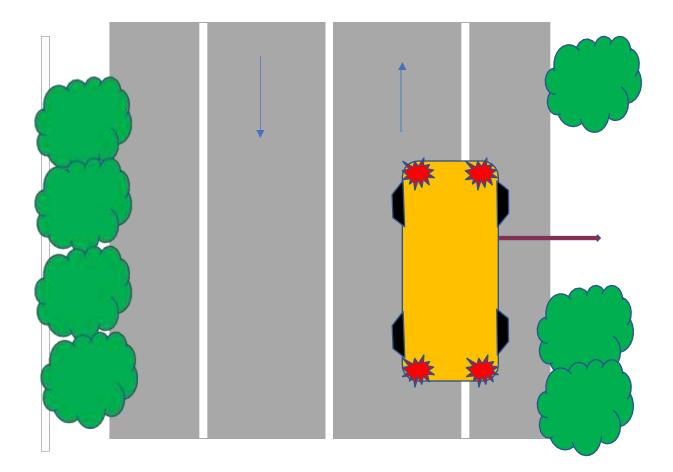
Proper placement of a bus on a paved roadway with a paved shoulder and students are not crossing the roadway
