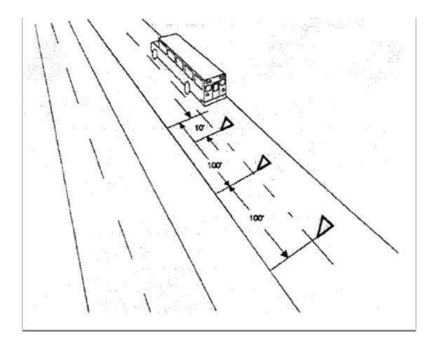
When placing the triangles, hold an assembled triangle toward the oncoming traffic. This enhances safety by increasing visibility for other drivers (especially at night).
