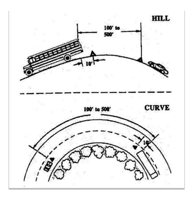
Reminder: If the line of sight is obstructed due to a hill or curve, move the rearmost triangle to a point giving adequate warning.
