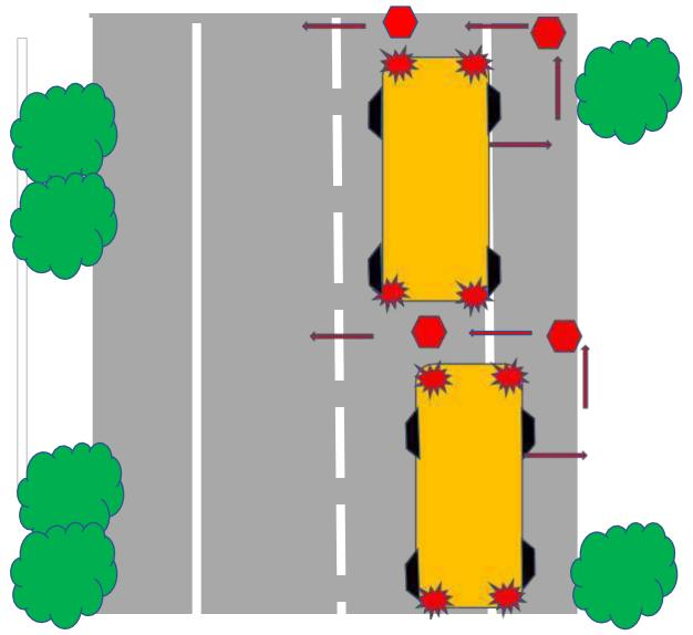
Proper placement of a bus on a paved roadway with a paved shoulder and students are crossing the roadway
